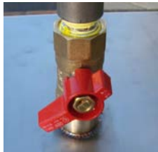
Main Trimmer Valve
